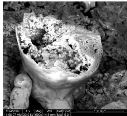
Pho. (6) SEM image of a pit formed on the iron surface during immersion the artifacts inside the seawater and before the reduction treatment.
