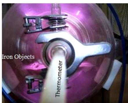
*pho. (2) Plasma thermometer and the Pyrex tube during reduction of marine iron artifacts by 100% hydrogen gas with violet color*
